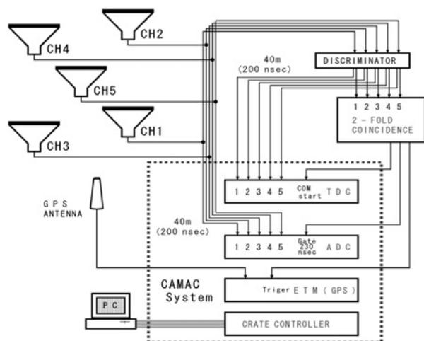
Figure 2. Block diagram of Hirosaki AS-Array II.
