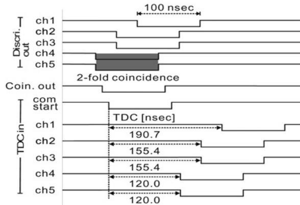
Figure 3 – 2. Timing chart of 2 fold coincidence. In the case of incidence from northwest.
