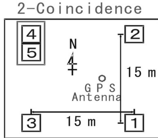
Figure 1. The counter arrangement of Hirosaki AS-Array II. 1 to 5 are fast timing scintillation detectors of area  $0.25m^2$  each. The triggering requirement is two fold coincidences of FT detectors No.4 and No.5.
