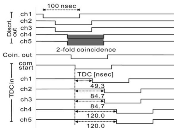
Figure 3 – 3. Timing chart of 2 fold coincidence. In the case of incidence from southeast.
