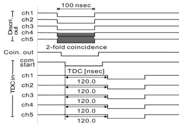
Figure 3 – 1. Timing chart of 2 fold coincidence. In the case of incidence from right above.
