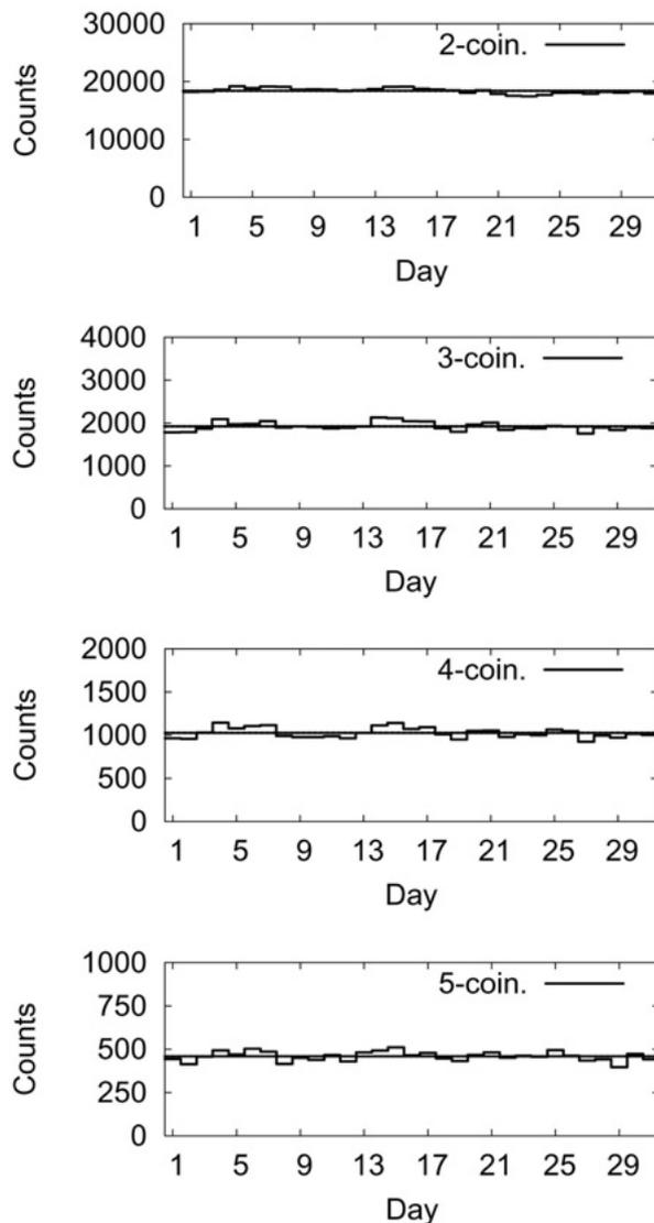
Figure 5. Trigger rate per day in the cases of 2 ~ 5 fold coincidence during 33 days.
