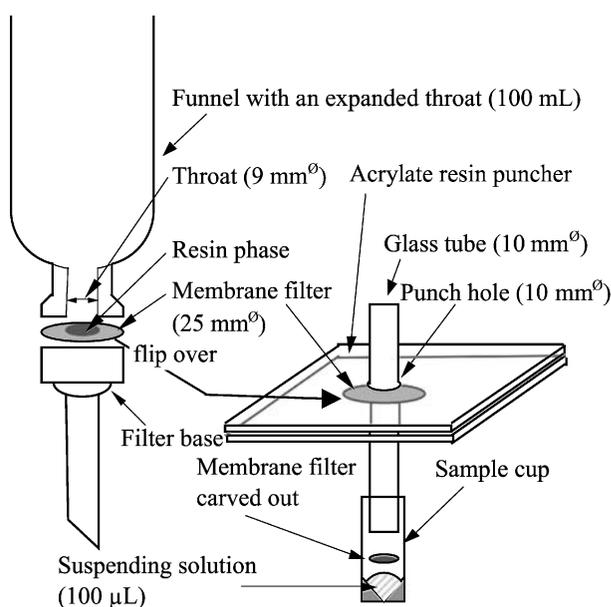
Fig. 1. Filtration apparatus and a purpose-built acrylate resin puncher
