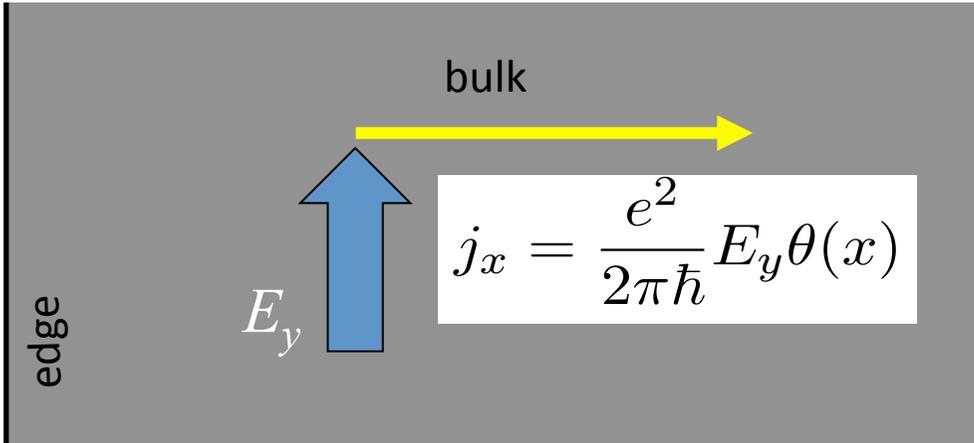
The diagram shows a gray rectangular region representing a quantum Hall system. The left edge is labeled 'edge' and the top boundary is labeled 'x=0'. A blue arrow labeled  $E_y$  points vertically upwards from the edge. A yellow arrow labeled 'bulk' points horizontally to the right. A white box contains the equation  $j_x = \frac{e^2}{2\pi\hbar} E_y \theta(x)$ .
