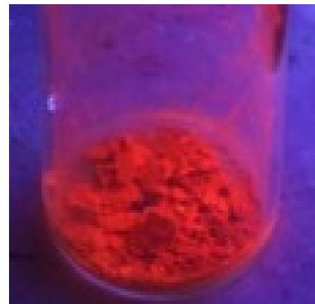
1-Benzothiazolyl-2-hydroxytryptanthrin (**T2OH1BT**) was synthesized as an excited state intramolecular proton transfer (ESIPT) fluorophore. In the solid state, the keto tautomer emission via ESIPT at 631 nm was observed, whereas the enol tautomer emission at 440 nm was observed.
